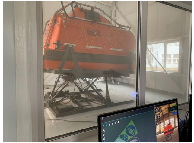
FFLBS Free fall lifeboat simulator
